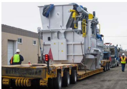
On its way to Mexico: The StrikoMelter HS-N melting furnace for cylinder block was manufactured in Michigan by StrikoWestofen America and transported directly to its final location.
